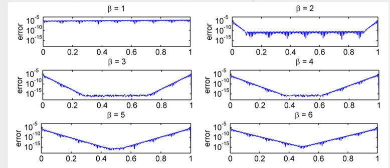
**Figure:** Error profiles over the interval  $[0, 1]$  for increasing  $\beta$ , with target function  $f(x) = e^x - (1-x) - ex$ . This function satisfies the boundary conditions only for  $\beta = 1$ . Note how error begins spreading towards the interior when  $\beta = 2$ , yet error continues to decrease in the interior. The interplay between these two phenomena indicates that there is an optimal choice of  $\beta$ , at least for a subregion of the domain.
