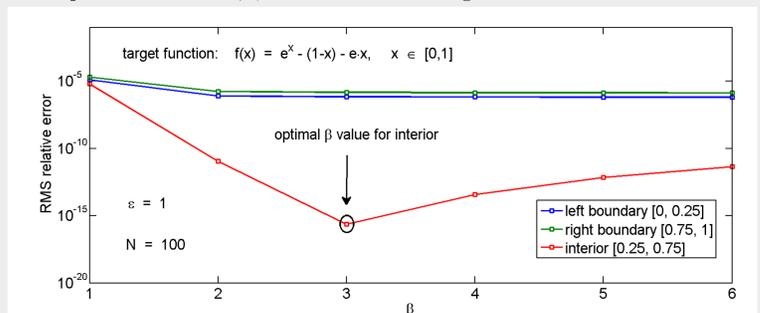
**Figure:** RMS error for interior and boundary regions. When we consider the interior of the interval separately from the boundaries, we observe that there is an optimal  $\beta$ .
